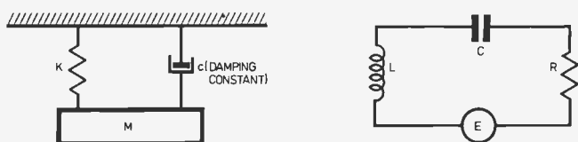
Fig. 4.1. The mechanical and electrical equivalent circuits for damping.
