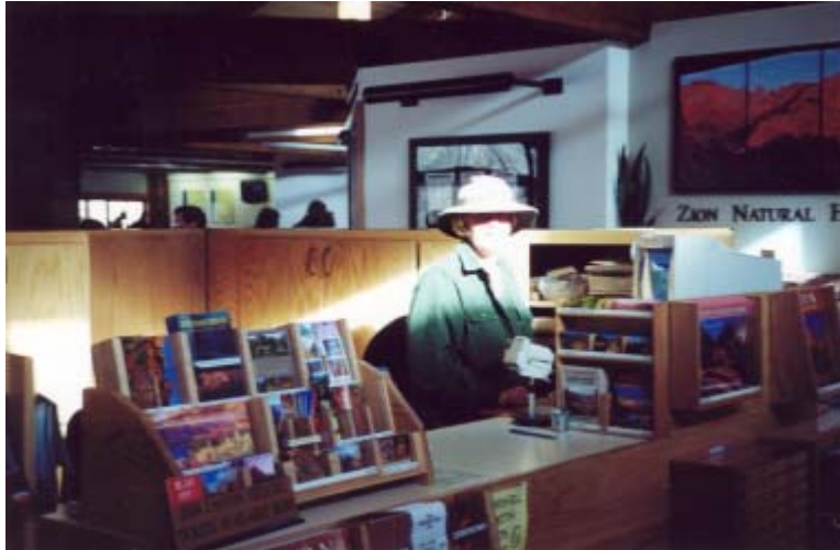
Figure 6-26 NPS bookstore checkout counter glare from clerestories
