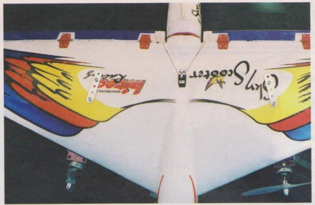
ABOVE: View of the top of the model showing the bolted attachment of the engine pylons. These engines can be easily removed so the model can be flown conventionally on the single central engine.
